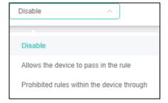
Select the rule of IP Filtering, default is Disable. Whitelist: Allow the devices to pass in the rule Blacklist: Prohibited rules within the device through
